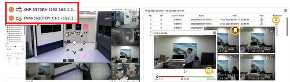
Live monitoring and PTZ control
